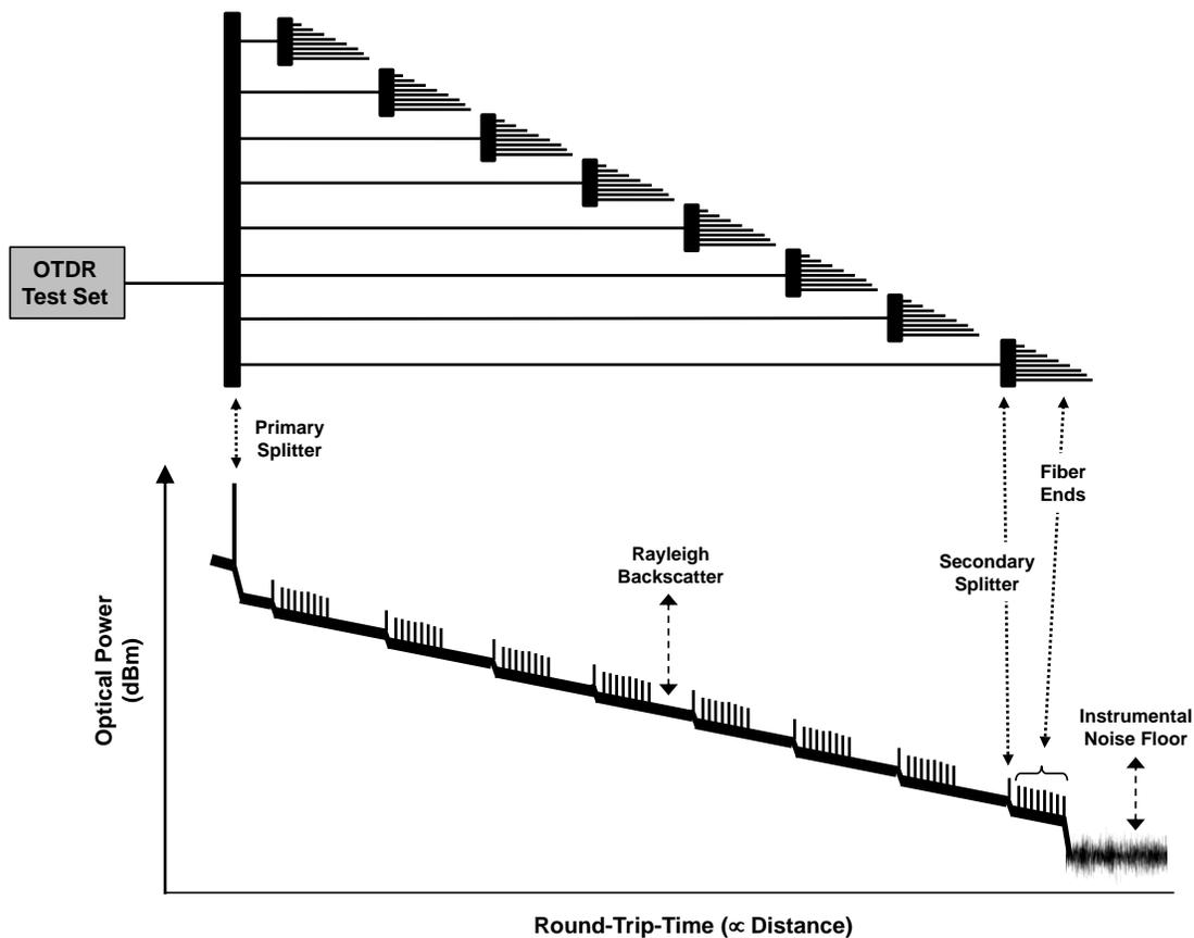
**Figure 12** – OTDR characterization of a 1x64 PON.
