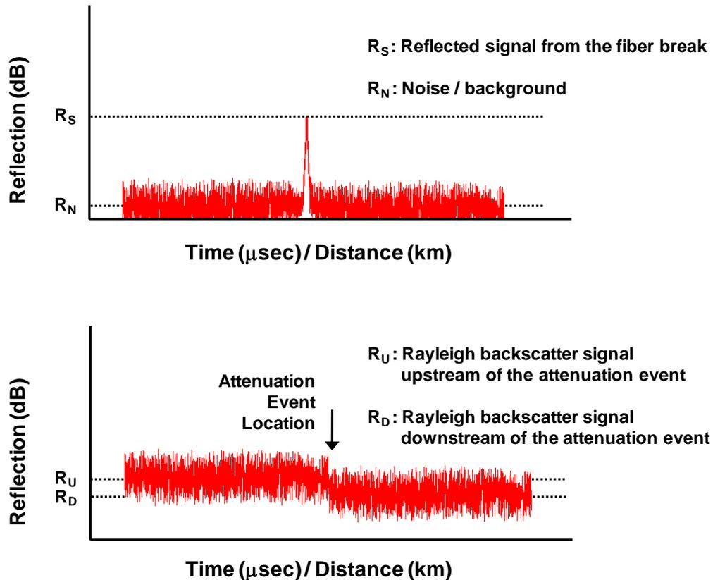
**Figure 14** – Detection criteria for fiber faults.
