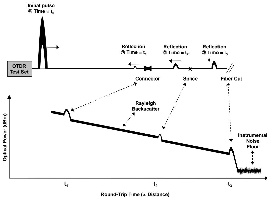
**Figure 11** – OTDR characterization of a point-to-point link.
